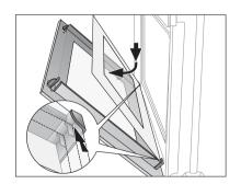
2. Take hold of the door trim (B) at each side, position it on the inside edge of the door and plug the door trim (B) into the upper edge of the door.
